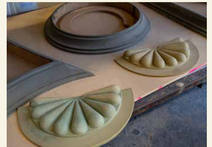
This page: At Liquidstone in west Auckland, workers spent months reconstructing the Hayman Building's pediment, removed decades ago as an earthquake risk. The new version was designed using archival photographs and built from glass-reinforced concrete. Photos by Joe Hockley.
