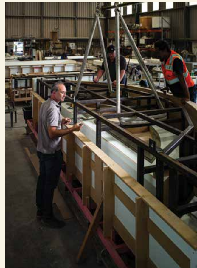
This page: At Liquidstone in west Auckland, workers spent months reconstructing the Hayman Building's pediment, removed decades ago as an earthquake risk. The new version was designed using archival photographs and built from glass-reinforced concrete. Photos by Joe Hockley.
